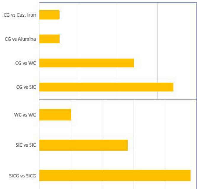
Maximum PV allowed for sealing face combinations
